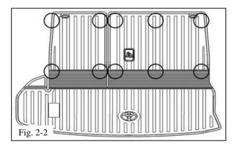
(d) Rub/massage areas of cargo tray shown to ensure proper velcro attachment to seatback before actuating rear seats up (Fig. 2-2).
